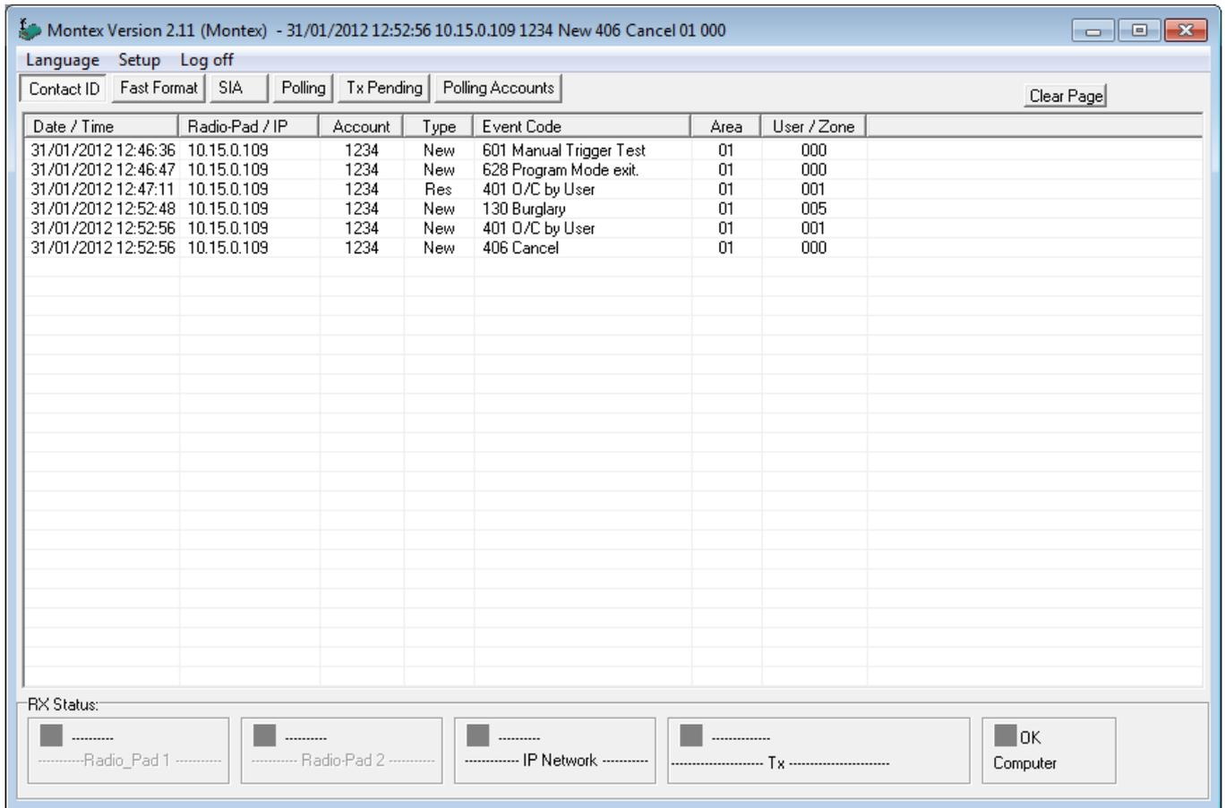
The status lights at the bottom of the screen indicate activity from the radio pads, ComIP or the Alarm Management Software (Tx). The 'OK Computer' status light indicates correct connection with the Alarm Management system.
